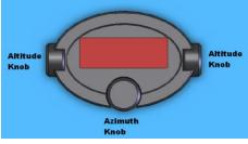
Rotating any of the two knobs adjusts movement in altitude direction or scrolls in the menus. Pushing the left knob toggles between the operation screen and the menu system. Pushing the right knob stops both motors (except tracking).
