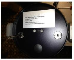
Adjustments screws are placed below a metal plate inside the mount head. There are also 4 screws holding this plate – they are not to be touched.
