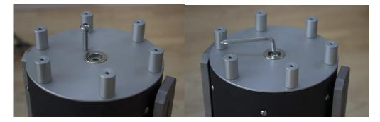
Tighten firmly with enclosed Allan Key - do not over-tighten.
