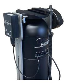
The mount must be powered up and aligned using the handpad. Now power up the Nexus adapter and connect the Phone/tablet and start using the Skysafari app. See the Nexus II user manual for all the details (can be downloaded from <u>https://www.astrodevices.com/Products/NexusII/index.html</u>).
