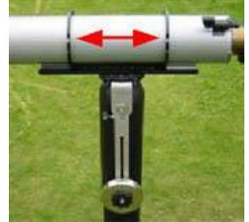
Now the counter weights are balanced. Loosen the altitude hand screws and point the telescope 60-80 degrees upwards. Now the counter weights can be positioned where the balance is right. Place the two counter weights in approximately the same height.
