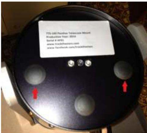
3. Remove the two plastic caps. Can be lifted with the sharp edge of a knife.
