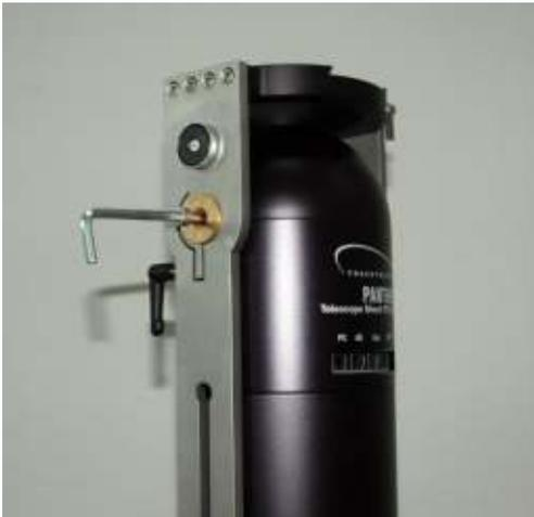
Release the two altitude clutch handles and rotate the counterweight arms to a horizontal position.
